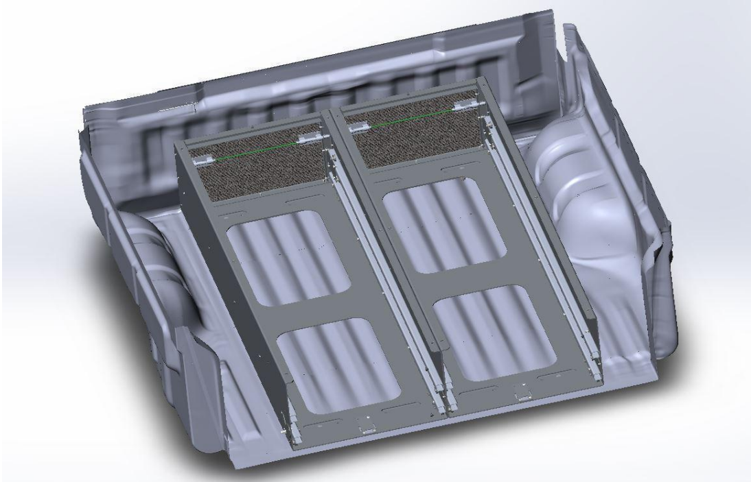
Figure 6: Drawer System Frame on Vehicle Load Bin
