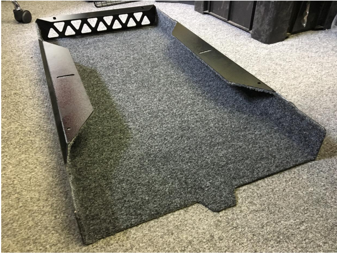
Figure 10: Main Carrier Body Carpeting
